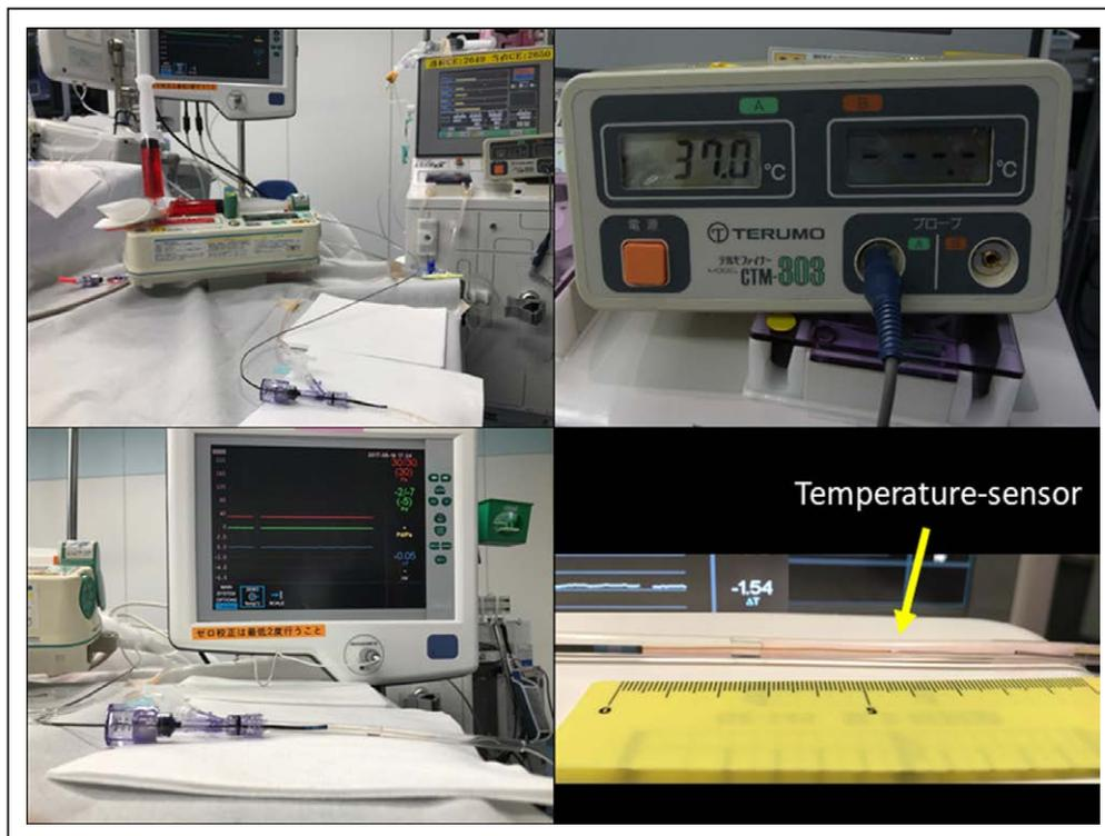
**Figure 4.** Experimental equipment for simulating the mixture of room temperature saline (red colored, 20 mL/min, 25°C) infused from the end-hole catheter and pulsatile flow of body temperature saline (pulsation flow auxiliary circulation system, 150 mL/min, 37°C) within a model composed of silicon tube, infusion pump, and dialysis machine. The sensor of a pressure–temperature sensor-tipped wire was placed 5 to 6 cm distal to the end-hole catheter (bottom right).
