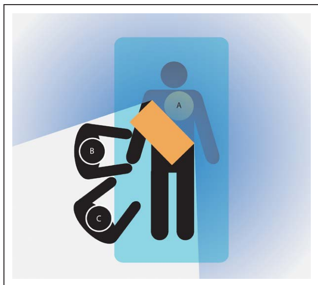
Figure 1. Position of the absorbing shield, placed on the patient, between the image intensifier (A), the primary operator (B), and occasionally the secondary operator (C).
